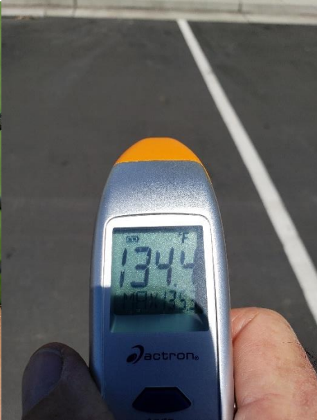
Artificial Turf Morgan Hill – 141.8 F Asphalt Morgan Hill – 134.4 F
