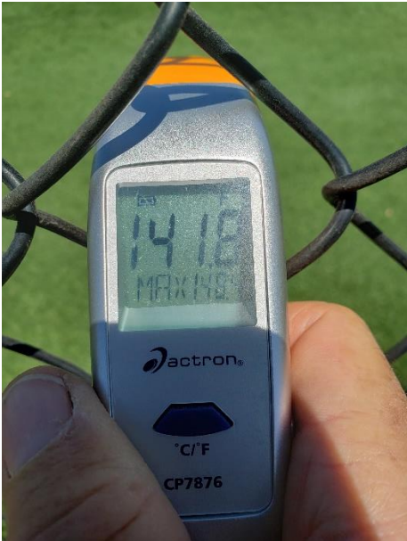
Artificial Turf Morgan Hill – 141.8 F Asphalt Morgan Hill – 134.4 F
