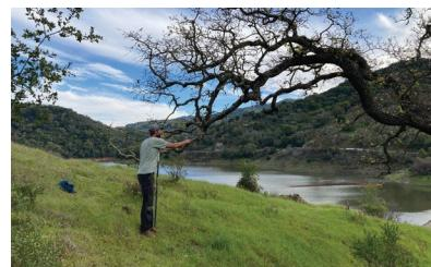
Lichen sampling at Guadalupe Reservoir for analysis to determine atmospheric mercury deposition.
