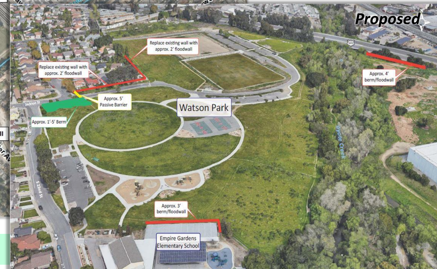
Figure 4.17. Proposed flood risk reduction improvements at Watson Park and immediately upstream of Highway 101
