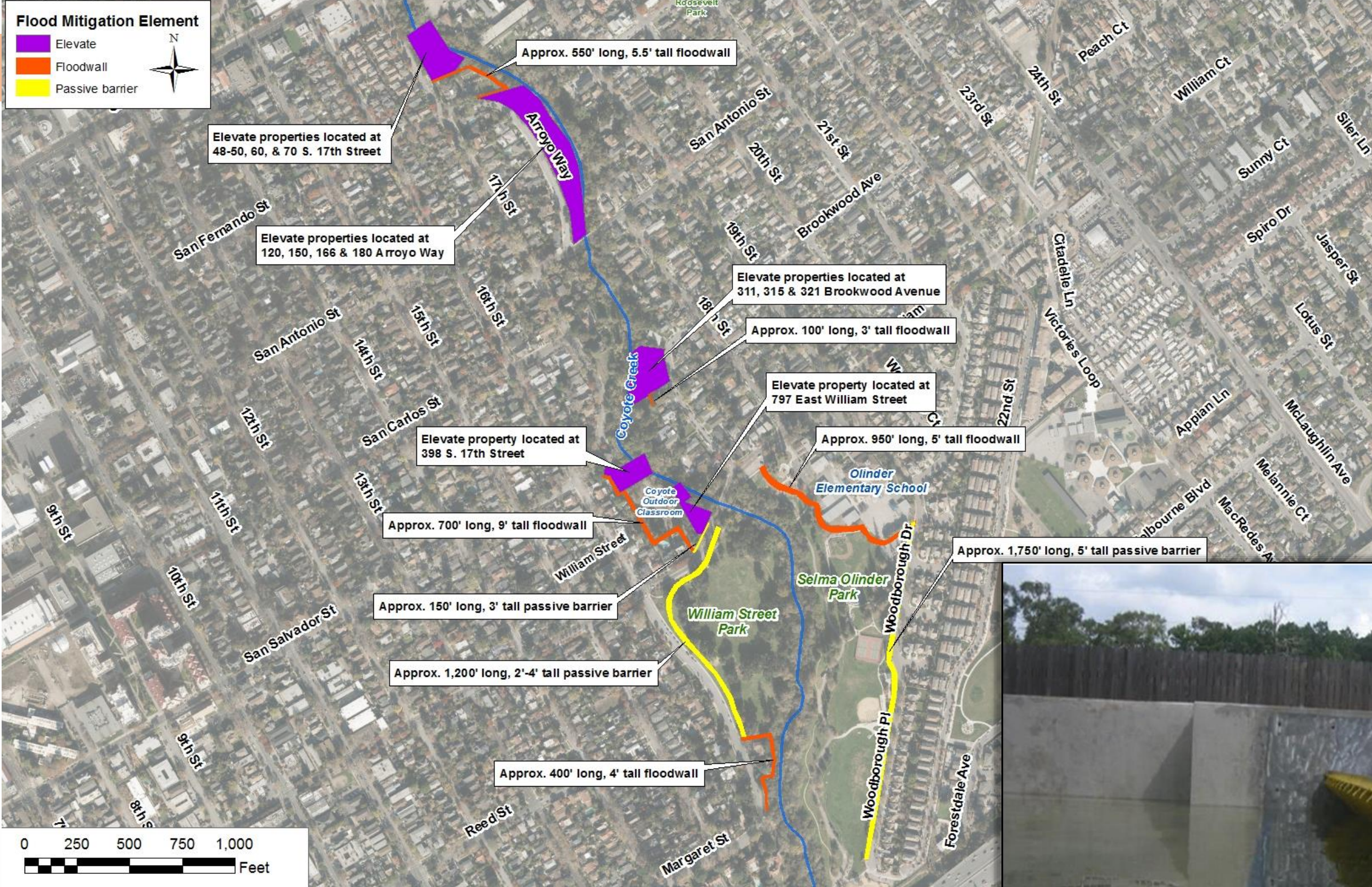
Figure 4.26. Plan View of Reach 7 – East Santa Clara Street to Highway 280 – For Feasible Alternative E3 & F3
