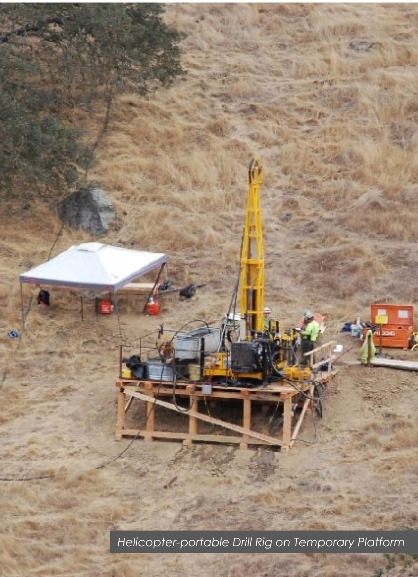
Helicopter-portable Drill Rig on Temporary Platform
