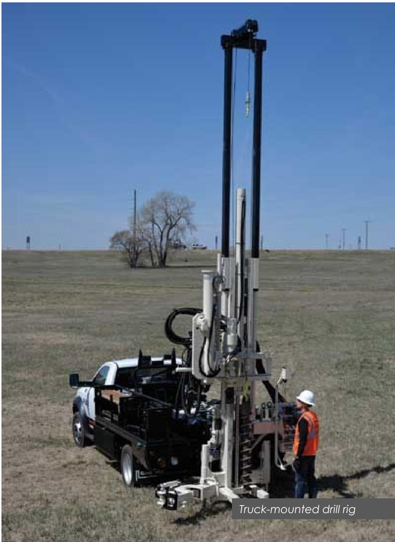
Truck-mounted drill rig
