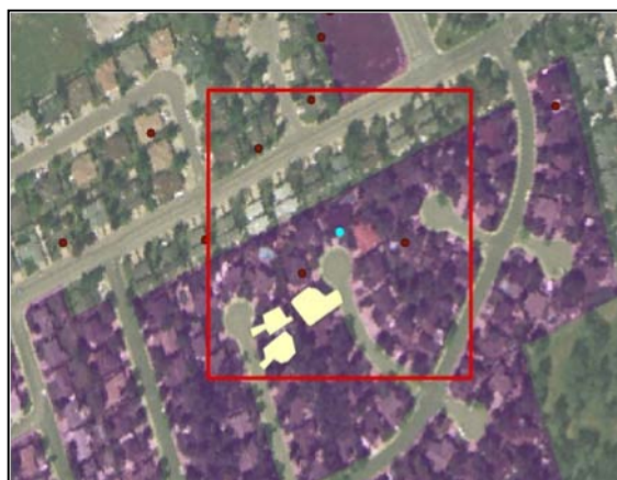
Figure 2. Analysis Box. An example of a randomly generated sample point around which a 40,000 sq. meter box, approximately 9 acres, was constructed. All impervious areas within the LUC on which the point was found and within the box were digitized.
