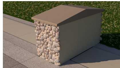
This is a rendering of a wiper wall. Once installed, it will connect sections of passive barriers and work as a seal to keep floodwater away from the neighborhood.
