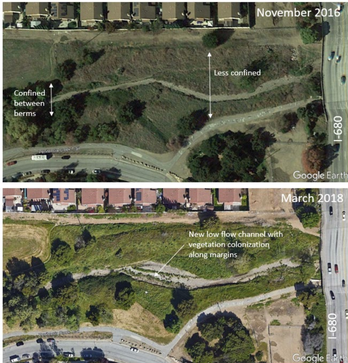
Figure 9 Google Earth imagery from before and after the January-February 2017 storm events just downstream of the I-680 crossing in Reach 3
