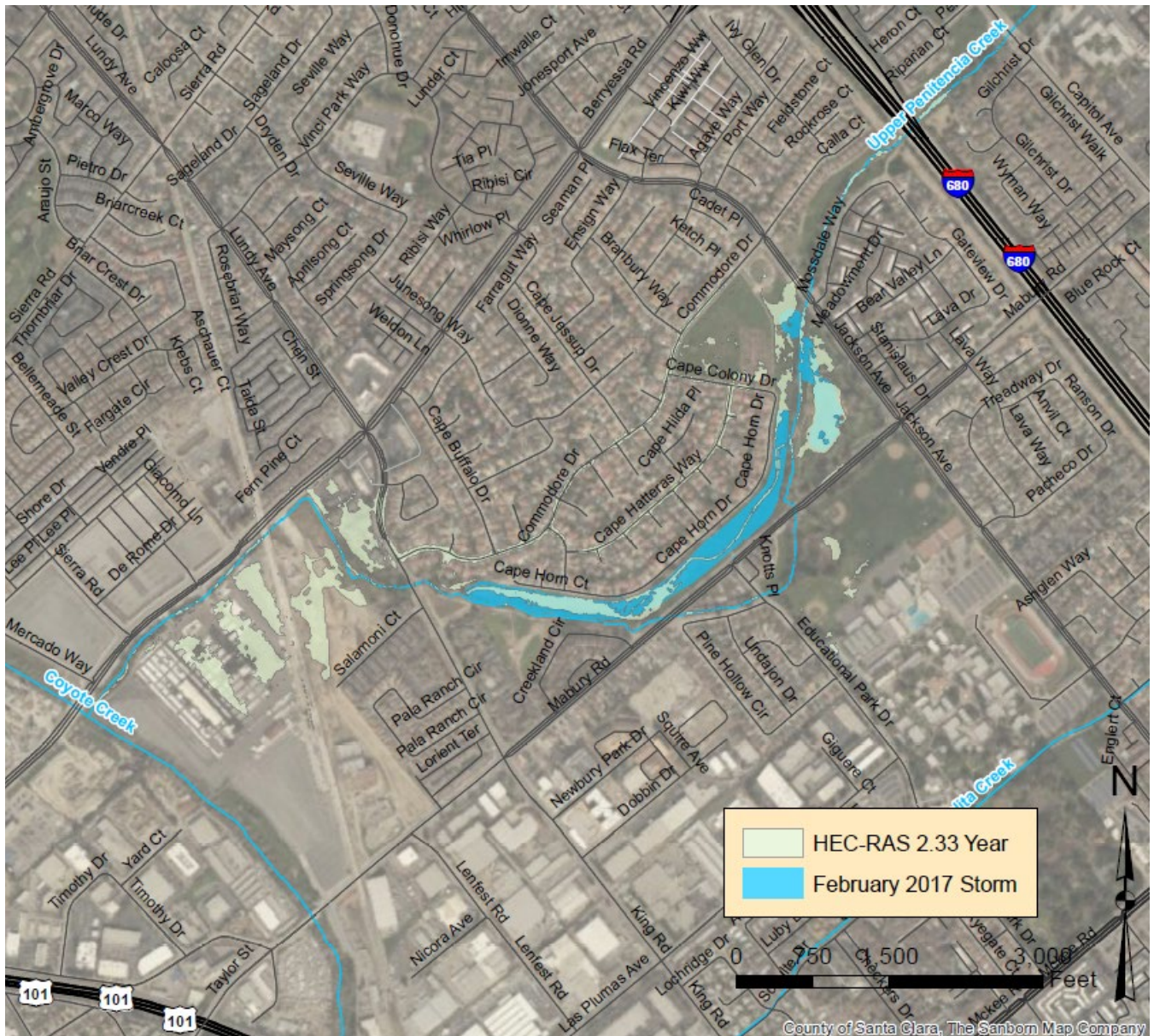
Figure 4 – Comparison of February 2017 storm vs. HEC-RAS output for 2.33-year Storm
