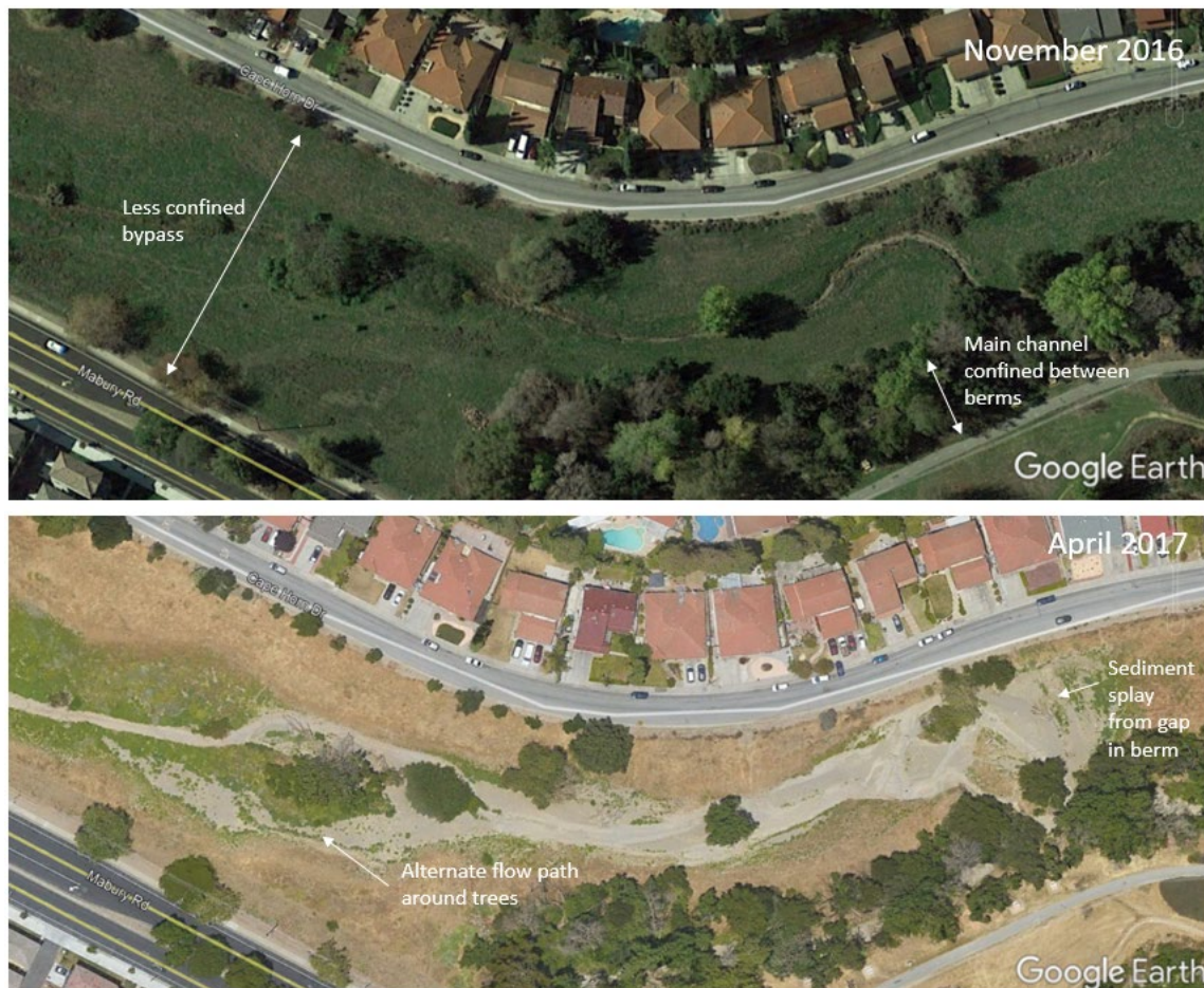
Figure 8 Google earth imagery from before and after the January-February 2017 storm events in the Reach 2 bypass between the Mabury Road crossings
