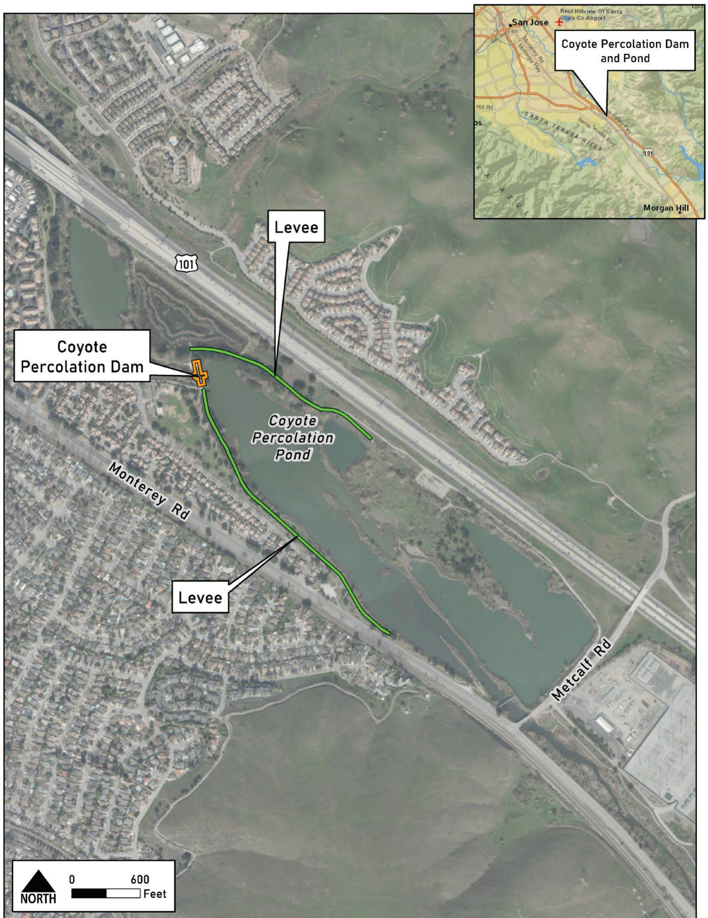
Figure 1. The Coyote Percolation Dam is located 11 miles downstream of Anderson Dam and is used by Valley Water to impound water within the 32-acre Coyote Percolation Pond for the purpose of groundwater recharge.
