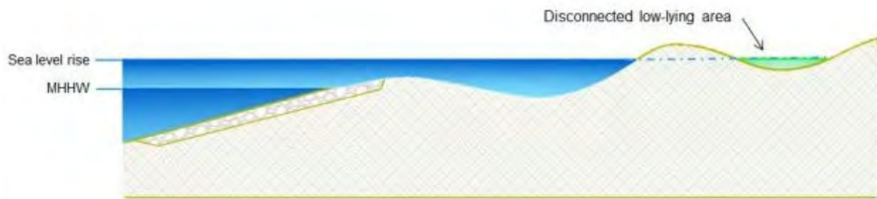
Figure 8-4. Example Shoreline Cross Section Showing Disconnected Low-lying Area
