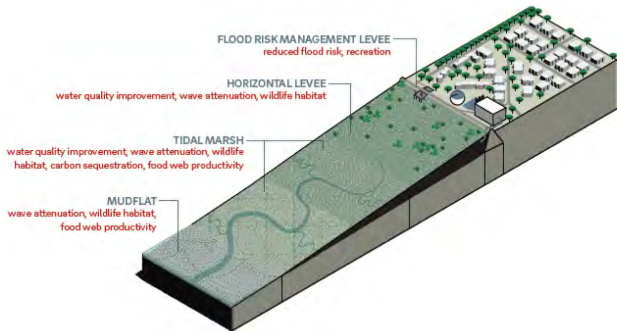
Figure 3-5. Horizontal Levee Concept
