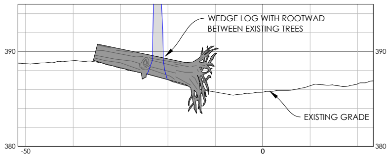
B SECTION AT LOG PLACEMENT SCALE: 1" = 10' VERT X2
