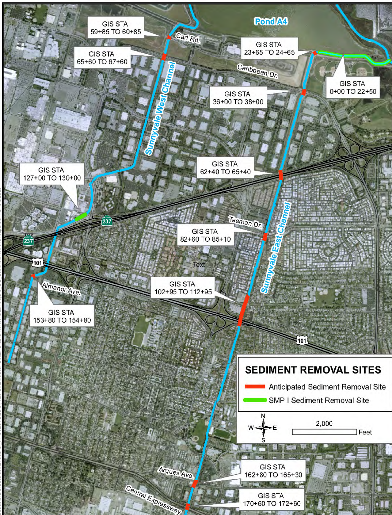
Figure C-2 Sediment Removal Sites Downstream from Central Expressway
