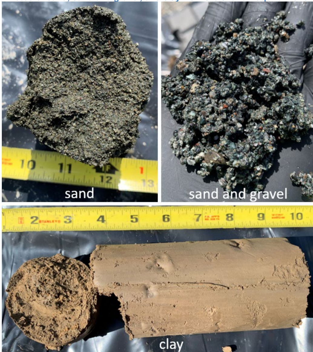
Figure 2-3. Photos of sand, sand and gravel, and clay from the shallow aquifer zone
