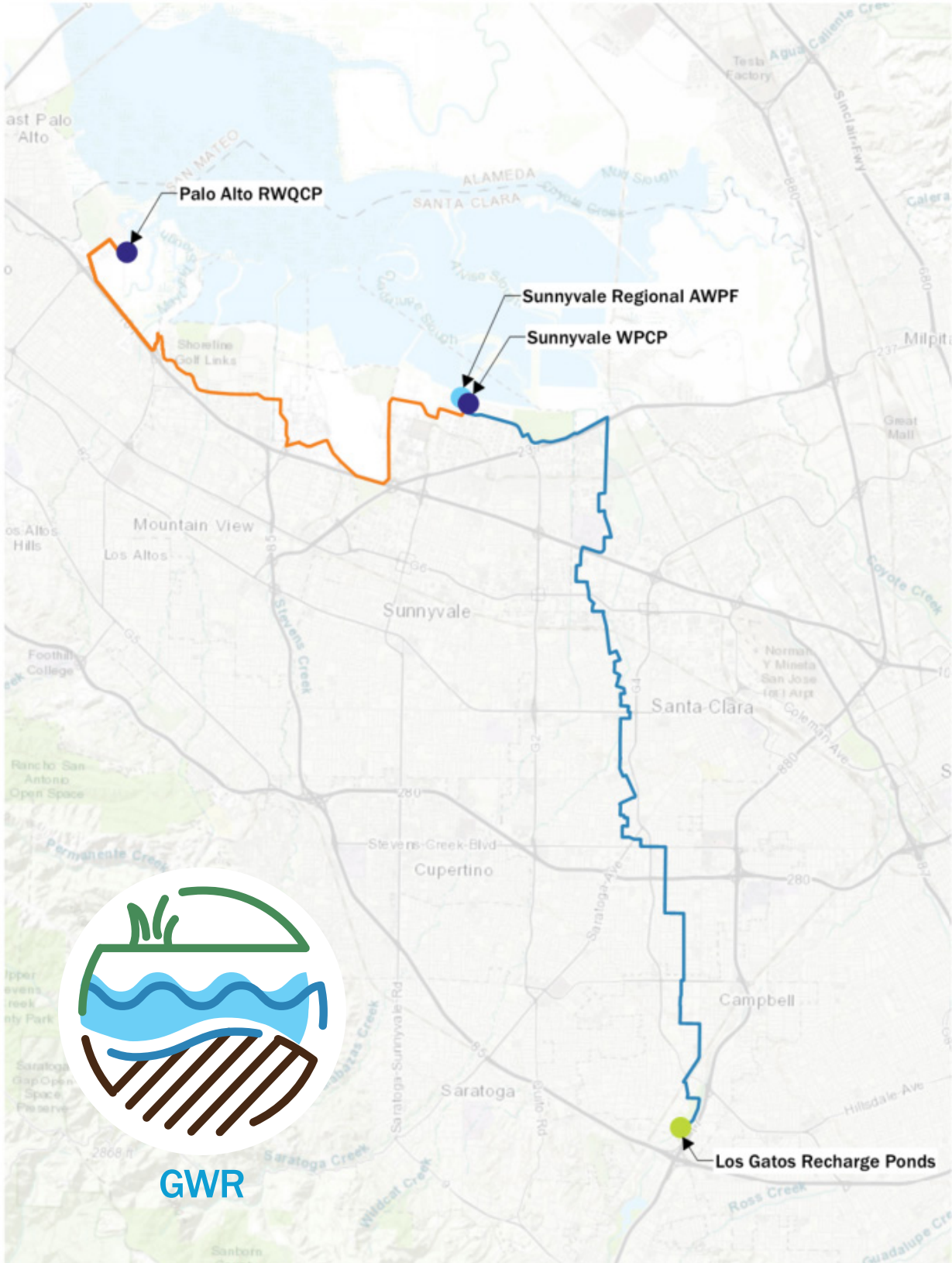
Figure 6-5. Portfolio 2a: PA (+SV) GWR facility locations and pipeline alignments
