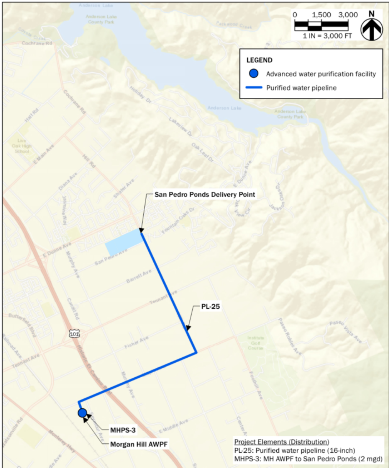
Figure 6-9. Facility locations and pipeline alignments for Morgan Hill Option 2 (Morgan Hill satellite AWP, GWR at San Pedro Ponds)
