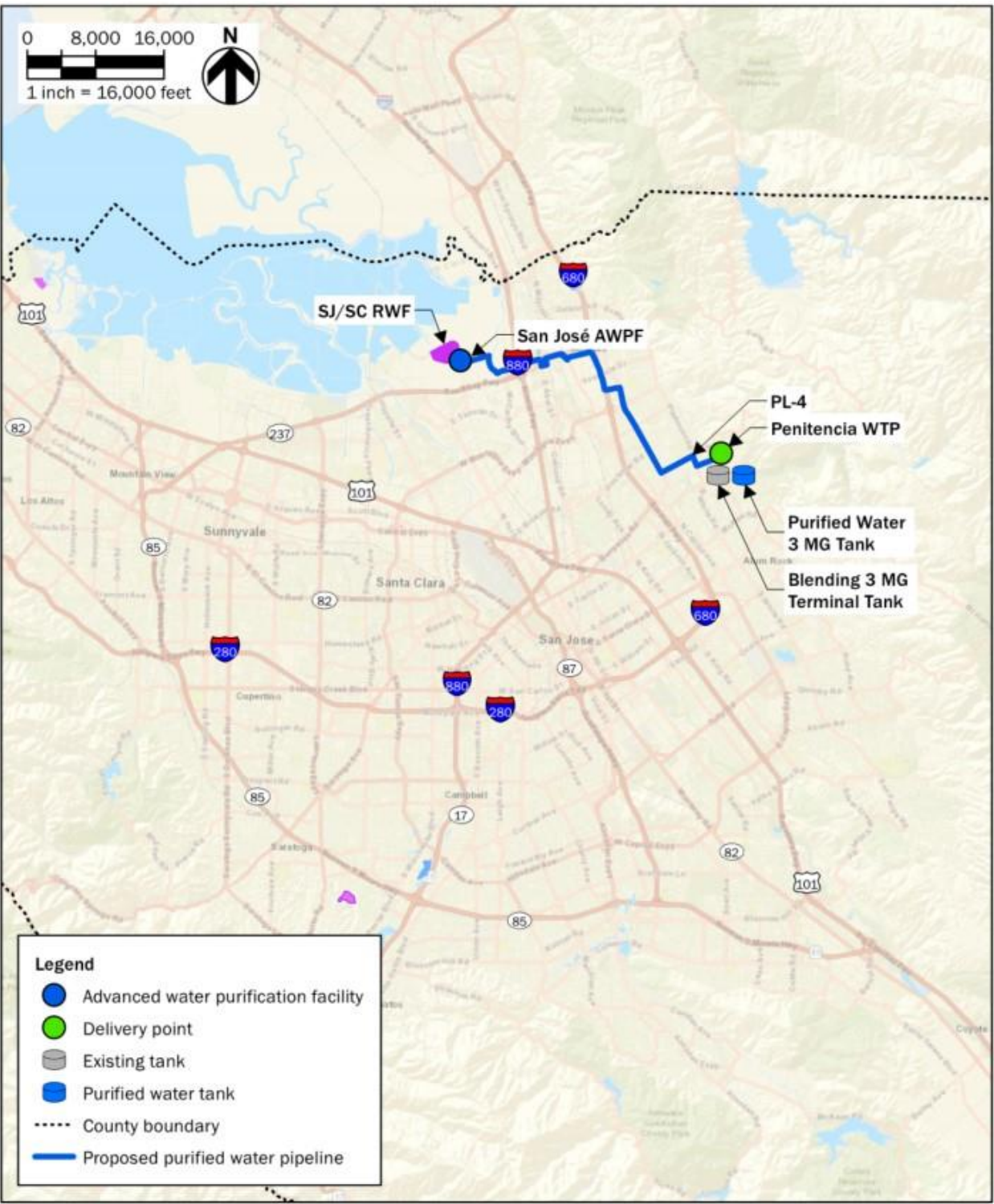
Figure 6-2. Facility locations and pipeline alignments for Portfolio 1b (San José AWPf, RWA at Penitencia WTP)
