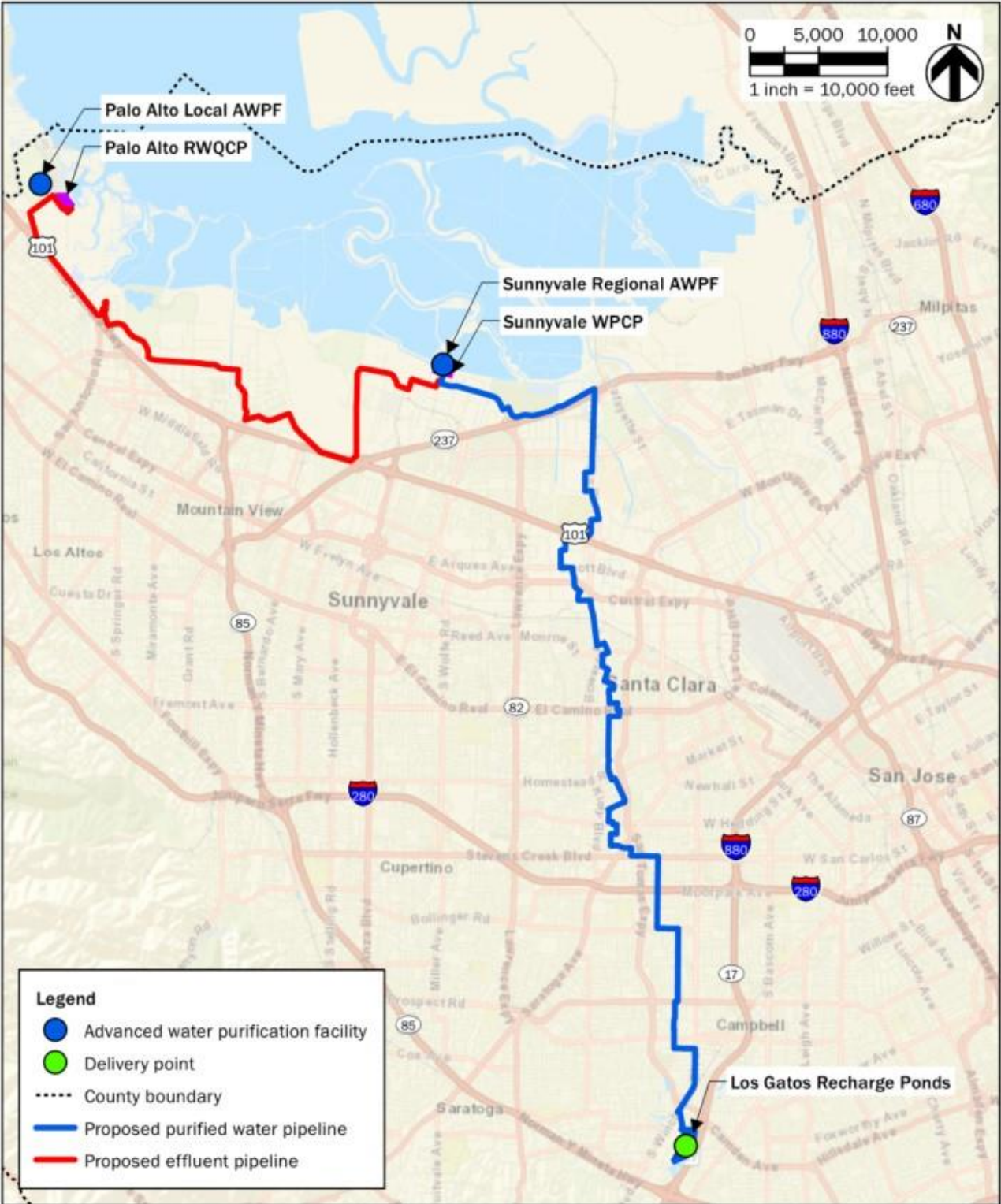
Figure 6-6. Facility locations and pipeline alignments for Portfolio 2b (combined regional AWP in Sunnyvale for GWR at LGRP)
