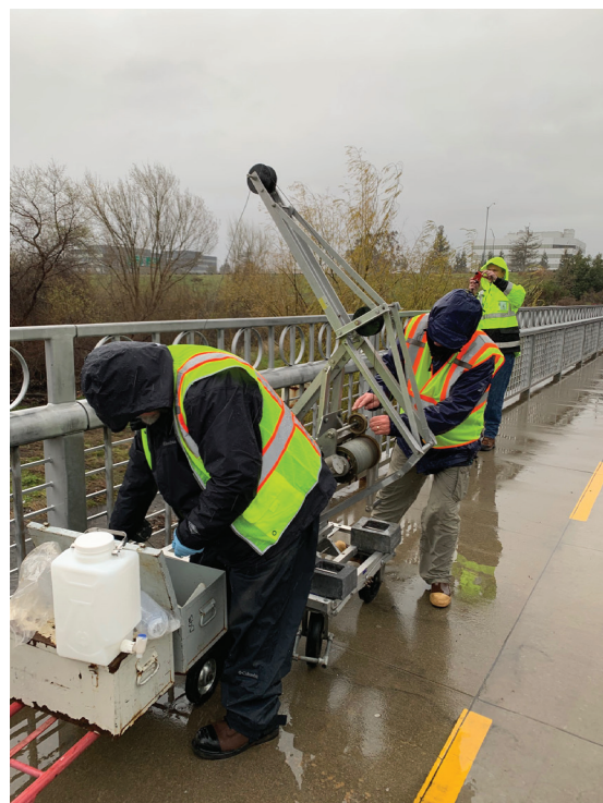
Sampling a Storm for Mercury at Guadalupe River.
